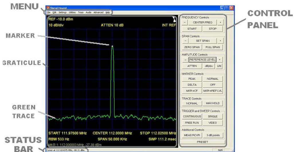
Figure 1 – The Signal Hound Graphical User Interface (GUI)
