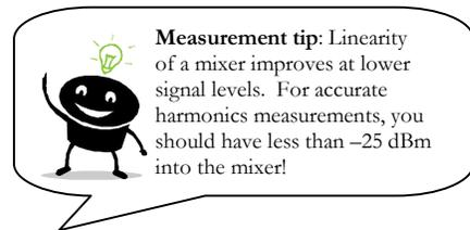
The mixers can typically operate with up to +0 dBm input, but keeping the input level -25 dBm or lower will greatly improve linearity.
